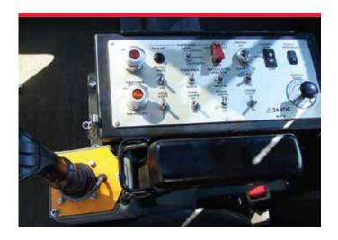
Electronic console with joystick workhead controls.
