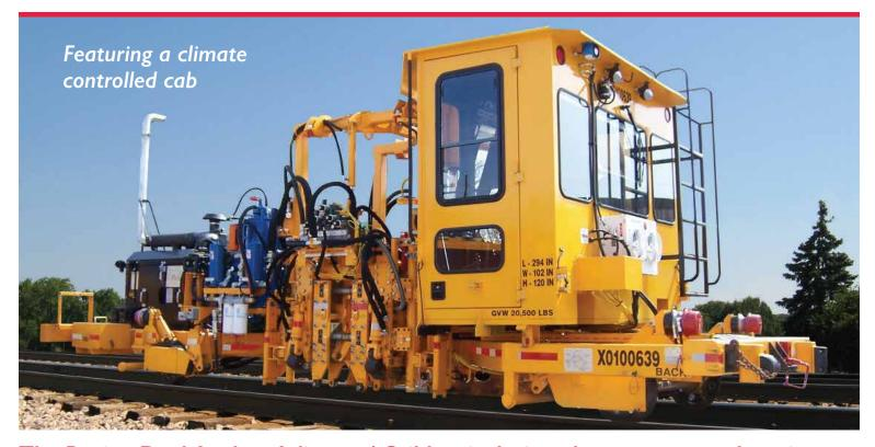
The Racine Dual Anchor Adjuster / Cribber is designed to squeeze anchors in full crib on one or both rails simultaneously. Can also be outfitted to straighten skewed concrete ties (with optional tools).
